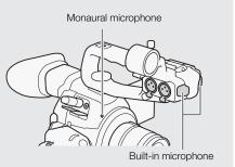
3 Plug the microphone cable into the desired XLR terminal (④) or the MIC terminal (⑤).
